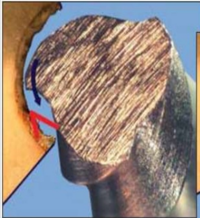
Fig. 26 The Hero file , with asymmetrical flutes, has a rake angle (red line angle of left image ) that is different from its cutting angle (red line angle of right image). The cutting angle is less negative than the rake angle and a better indication of its cutting ability.
